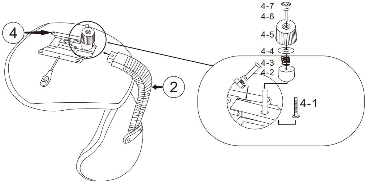
**STEP 6:** Put mechanism(4) on the gas lift(5), as instruction shown.
